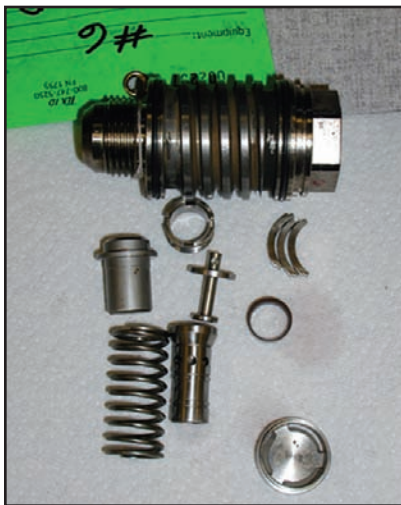
Inspection of the fuel check valves showed no or very little evidence of fuel coking after approximately 1300 total hours of operation — of which 300 hours were on attained or liquid fuel — with some 50 fuel changeover sequences completed.
