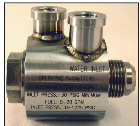
Shown is a single JASC liquid-cooled fuel valve prior to installation.
