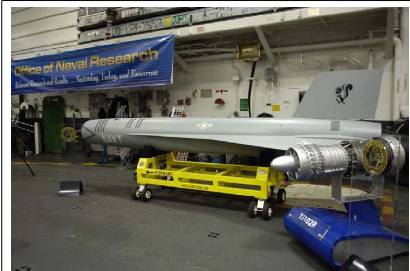
Pictured during Fleet Week 2006, a mock up of the RATTLRS vehicle and the YJ102R engine (which will power the RATTLRS vehicle) are on display. Noteworthy in the vehicle's overall shape is the design heritage drawn from the SR-71's engine nacelles and moveable inlet spike. Image courtesy ONR
